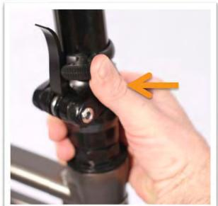
Lift the locking lever to the vertical position, securing the release button into the locked position.
