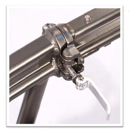
To unfold the frame, position the unlocked frame quick release perpendicular to the bike frame.
