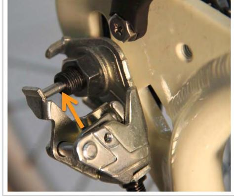
For a properly adjusted hub, this red indicator line will be evenly aligned with the threaded axle end.
