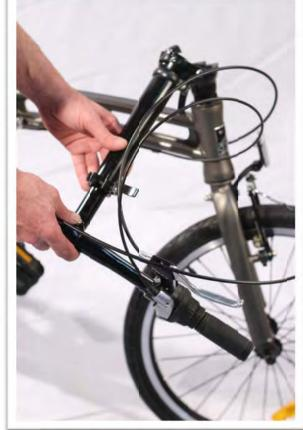
Please note, your handlebar extension has an imprinted minimum insertion or maximum extension marking. Do not adjust your handlebar extension beyond this marking.
