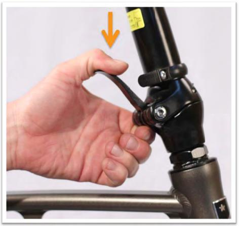
Next, firmly press the wedge release button to unlock the handlebar stem wedge. Once released, fold the handlebar stem to the side of the bike.
